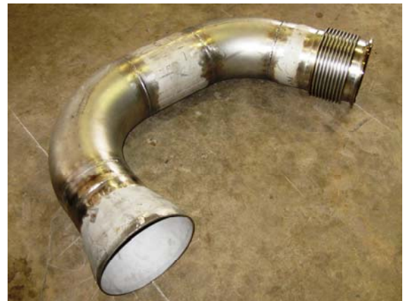
Small gas turbine exhaust piping with bellows
