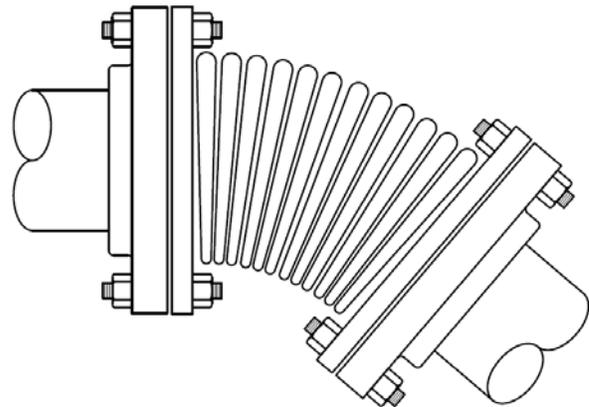
*The bellows takes away the flanges need to transfer bending forces*
