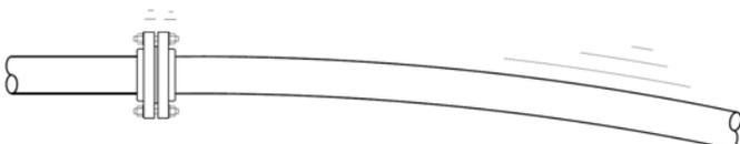
*The flange is designed to be as strong as the pipe in bending*
