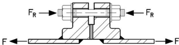
*Flange hub is designed to resist several bending forces*
