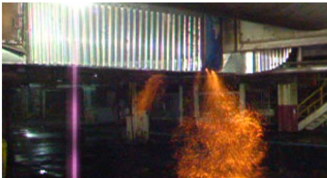
Coal dust igniting through tears in the fabric expansion joint
