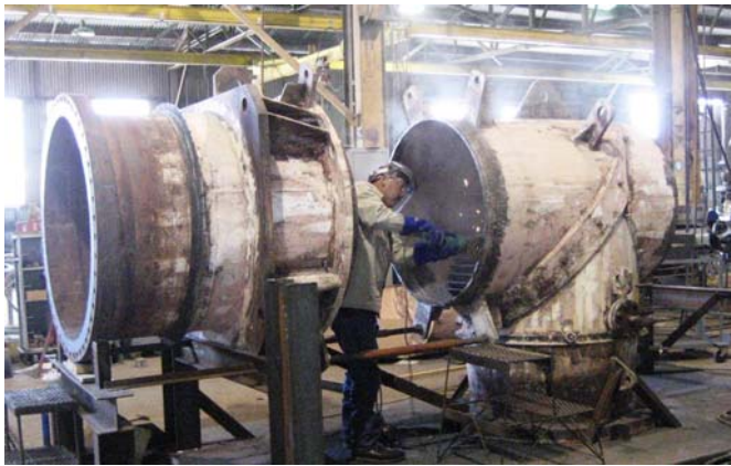
A stripped down cross-over with bellows removed
