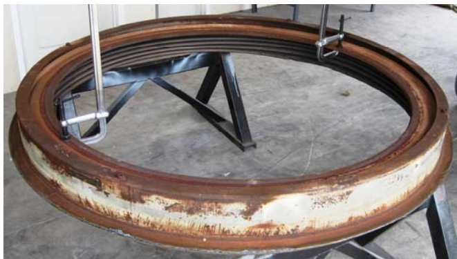
Old GE condenser seal with leaking metal bellows
