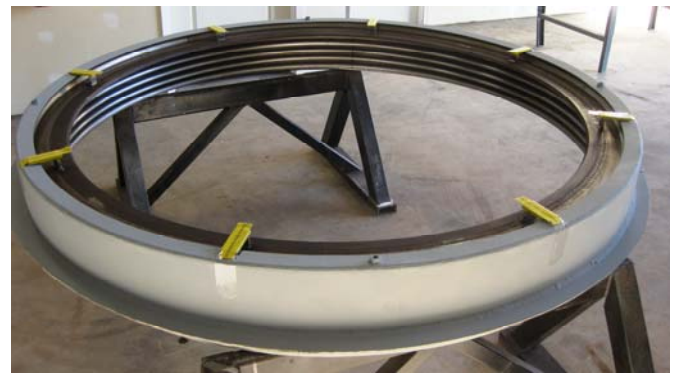
Refurbished condenser seal with new metal bellows
