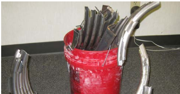
A 2-ply alloy 625 bellows failed after only 5 years in service
