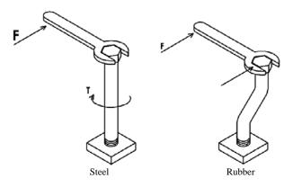
That's how a low lateral spring rate expansion joint works. The bellows can be designed with a low lateral spring-rate and, when used as a dual, still maintain the same torsional resistance.
