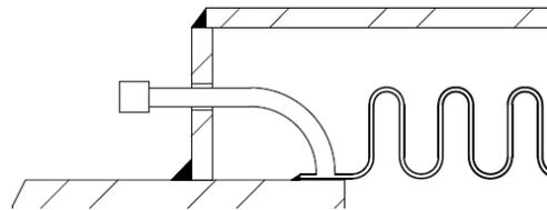
Also consider upgrading from stainless steel bellows to alloy 625 for better protection against chloride stress corrosion.
