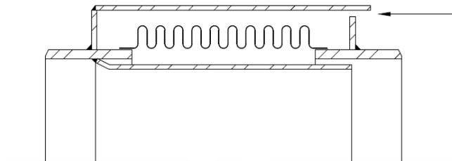
Look for signs of cover damage. Often the original designs had lighter covers (and liners) that would not hold up under the high flow velocities. Those fragments are lodged somewhere down in the condenser.
